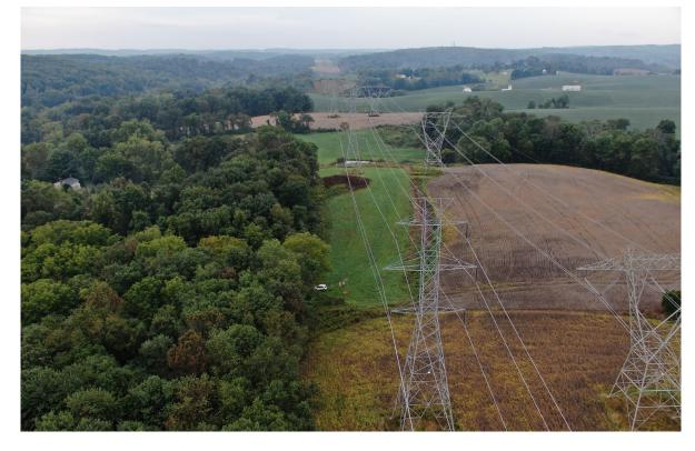
Utilizing drones to inspect Transmission structures allows for high quality inspection with less risk and a 60% reduction to O&M cost (~\$260k per year.)
