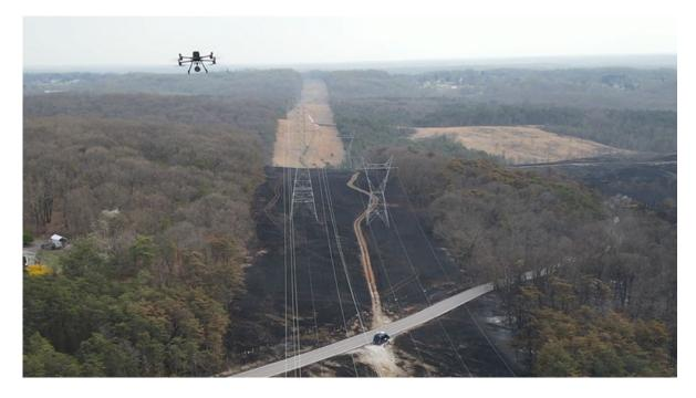
BGE along with Local FD and National Guard responded to a wildfire that had crossed over a Transmission ROW in Owings Mills and came in direct contact with tx structures and conductors. TEDS had requested the assistance of the Drone Team to assess any damage that may have occurred as a result of the fire & smoke.
